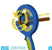
Continue winding sector of the harness by moving along the harness axis. Maximum recommended pitch should be equal to 3 tape widths.
