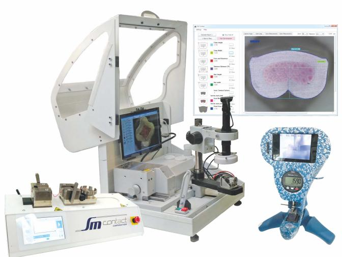
SKP 4000, SKB 4000, SKA 4000, SK 6000 – mobile & stationary, semi- and fully automatic micrograph laboratories EPT 1000 – motorized pull force tester CrimpiX - splice crimping height measurement tool Viso – measurement software
