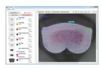
Captured image is measured with a help of special software – Viso 6.00. Operator chooses the parameters to measure, its reference values
